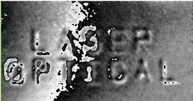
Shearography image: Resin enriched detail In composite panel
